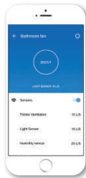
For electricians, installation is made simple through the App allowing you to choose intermittent or continuous ventilation; whether you would like the humidistat to trigger operation or not; and whether the overrun timer is required. No more fiddly switches and jumpers!
