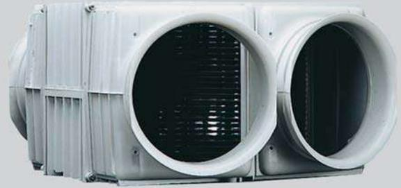
A 'stand alone' heat exchange module which will transfer up to 70% of the outgoing heat to incoming air. Polymeric construction with spigots to suit 200, 250 and 315mm Ø flexible ductwork.
