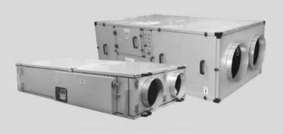
Mini and Midi Models are manufactured with a frameless construction from single skinned Aluzinc panels, internally lined with 90kg/m³ high efficiency acoustic and thermally insulating foam (fire retardant to BS476 Part 7 Class 1 & Part 6 Class O). Aluzinc panels allow for all units to be mounted either internally or externally as standard (IPX4). An optional inlet cowl is available for roof mounting applications if required.
