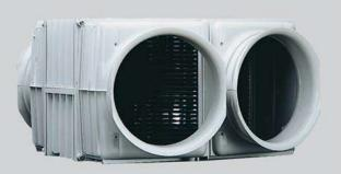
A 'stand alone' heat exchange module which will transfer up to 70% of the outgoing heat to incoming air. Polymeric construction with spigots to suit 200, 250 and 315mm  $\varnothing$  flexible ductwork.
